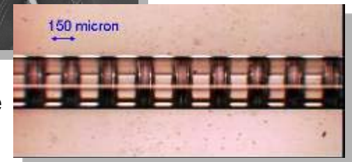
Grating in Sapphire Fiber (PSU)
